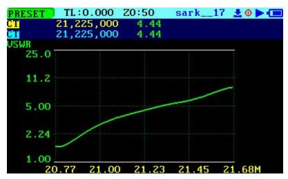
15 meters (21 to 21.45 MHz). The minimum SWR is off the low end of the sweep. The plot below shows a minimum SWR of 1.53 at 20.79 MHz. This low frequency is probably due to the proximity to the ground.
