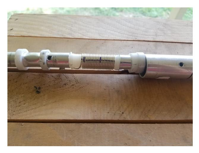
Note the hole in the tube to the right of the second white spacer from left and the hole in the trap shell on the right. A self tapping screw goes through the shell and is threaded into the inside tube. Several of these screws were loose, and, on one trap, the hole on the inside tube was stripped. Since the hole goes all the way through the tube, I rotated the shell so the screw went into the other side of the tube. Stripped hole problem fixed!
