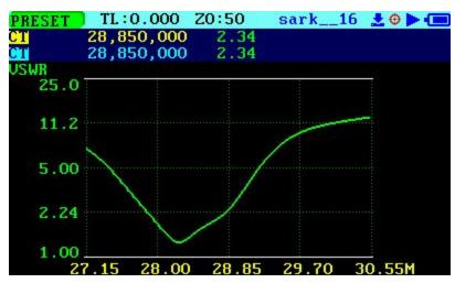
10 meters (28.0 to 29.7 MHz). Minimum SWR is 2.34 at 28.85 MHz.
